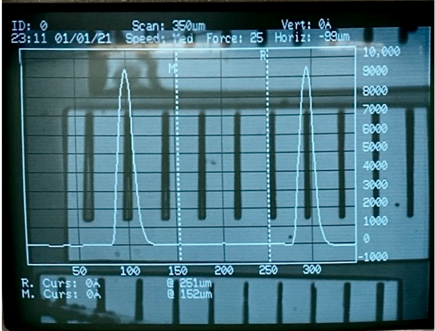
Profilometer scan of gate layer (y axis in angstrom, x axis is micron)
