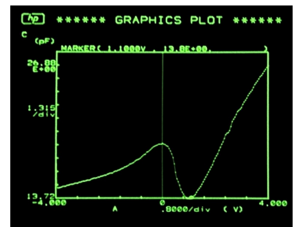
C-V showing V_{th} = 1.1V
